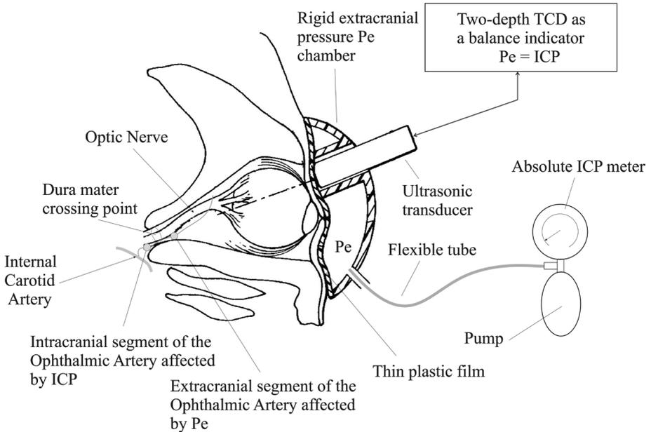
Fig. 1. Non-invasive two-depth TCD device components showing the relevant eye/brain anatomy. The ultrasound transducer of the Doppler subsystem is surrounded by an externally applied pressure chamber with a controlled external pressure ( $P_e$ ) source and measurement. (Reprinted with permission from Ragauskas et al. 2012.)
