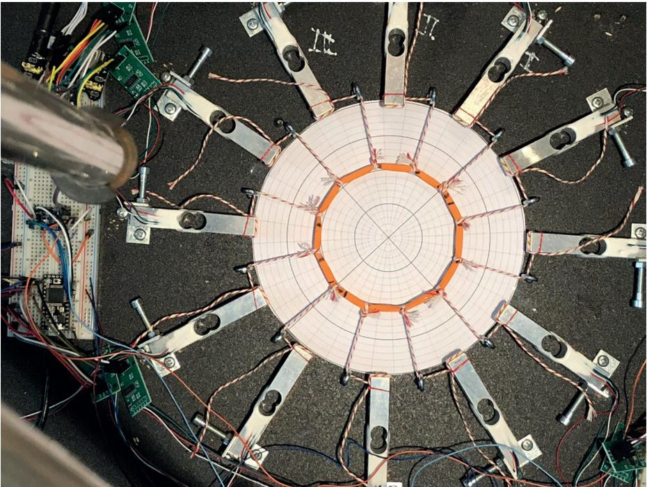
*Fig. 1.* Setup showing the arrangement of the load cells and the pre-stretched elastic band.
